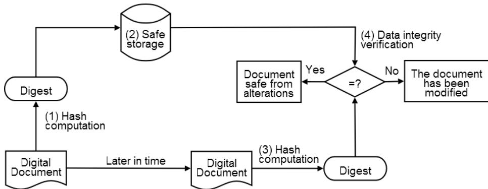
Fig 17.2 Assuring data integrity using Message Digests
