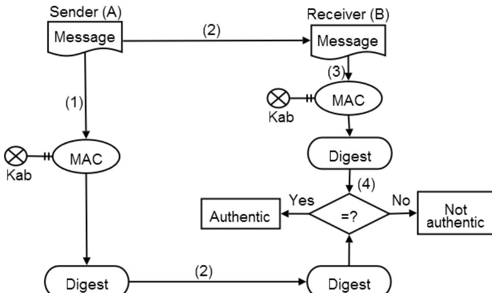
Fig. 17.3 Assuring data origin authentication using MACs
