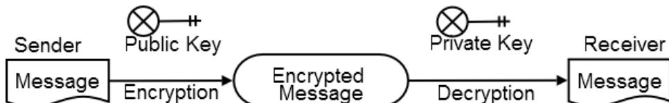
Fig. 17.5 Assuring confidentiality using asymmetric-key encryption
