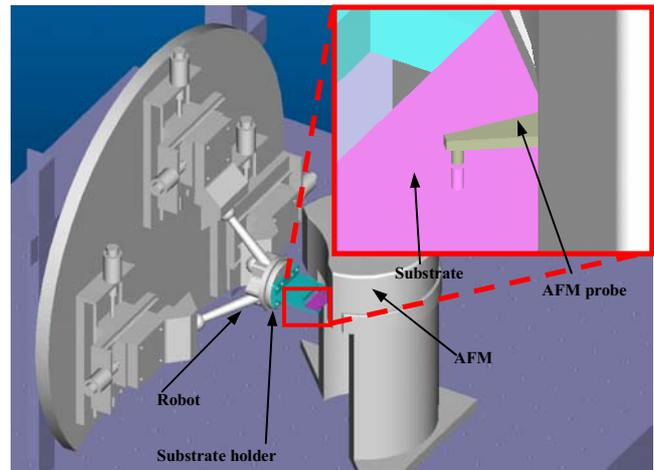
Fig. 1. The 3-D model of the micro-force measurement system – NANOROL.
