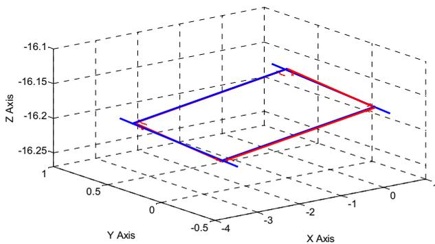
Fig. 10. The measurement data and the edges identification result when the orientation of the robot system is fixed to  $0.4^\circ$ ,  $-0.4^\circ$  and  $0.4^\circ$  respectively. (Blue lines: identified edges based on experiments; red lines: identified edges based on parameters estimation)
