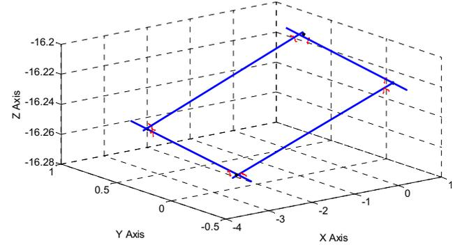
Fig. 9. The measurement data and the edges identification result when the orientation of the robot system is fixed to  $0.5^\circ$ ,  $-0.5^\circ$  and  $0.5^\circ$  respectively. (Red lines: scanning data; blue lines: identified edges; black asterisks: identified corners)
