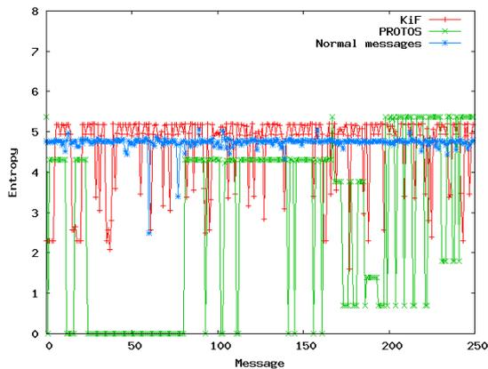
Fig. 7. The entropy of a fuzzing process on Linphone.
