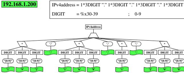
Fig. 12. Syntax tree representation of an IPv4 address.
