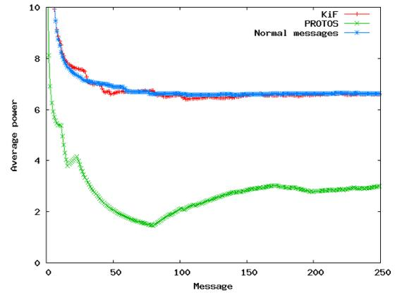
Fig. 6. Average power for two fuzzers on Linphone
