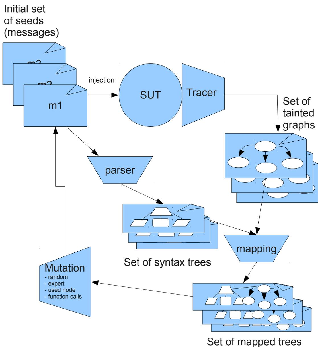
Figure 1: Fuzzing process by mutation using feedback
