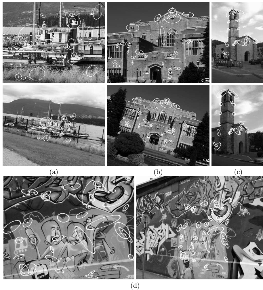
Fig. 7. For image pairs (a),(b) and (c) the top row shows the query images and the bottom row shows the most similar images in the database. For image pair (d) the left image is the query image and the right one the image in the database. The displayed matches are the inliers to a robustly estimated fundamental matrix or homography between the query image and the most similar image in the database. There are (a) 22 matches, (b) 34 matches, (c) 22 matches and (d) 33 matches. All of them are correct.
