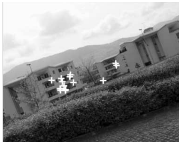
Figure 7: Example of images taken from different view points. There are 14 inliers to a robustly estimated fundamental matrix, all of them are correct. The estimated scale factor is 2.7.
