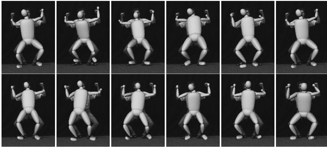
Figure 11: Minima of image-based cost functions: contour and silhouette likelihood. The model is initialized at one minimum (fig. 9, second figure) and search trajectories for other minima are initiated from there. The minima shown include ‘reflective’ (depth-related) ambiguities, incorrect edge assignments and singular ‘inside-silhouette’ configurations. More complex silhouette-based cost functions, as proposed in [39] can be further used eliminate some of the latter spurious minima (see text).
