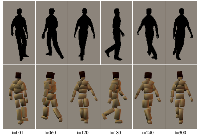
Figure 6. Some sample pose reconstructions for a spiral walking sequence not included in the training data, corresponding to figures 5(c) & (f). The reconstructions were computed with a Gaussian kernel RVM, using only 348 of the 1927 training examples. The average RMS estimation error per d.o.f. over the whole sequence is 4.1^\circ .
