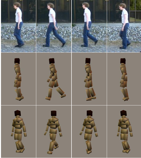
Figure 8. 3D poses reconstructed from some real test images (part of a sequence from www.nada.kth.se/~hedvig/data.html ). The middle and lower rows respectively show the estimates from the original viewpoint and from a new one. The last two columns illustrate limitations of our current system. In the third column, a noisy silhouette causes slight mis-estimation of the lower right leg, while the final column demonstrates a case of left-right ambiguity in the silhouette.
