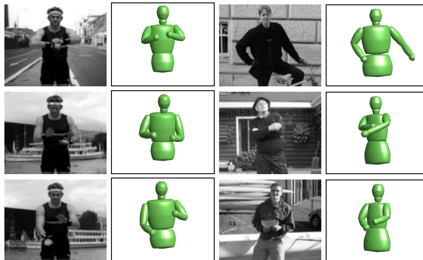
Fig. 6. Pose reconstructions on real unseen images. The first 3 images are taken from a test sequence in our motion capture dataset which includes similar gestures made by another person, while the last 3 are example images obtained using Google. The results on the real images are not very precise if overlaid on the images, but they do capture the general appearance of the subject's gestures fairly well. They would probably improve considerably given more training data for common gestures.
