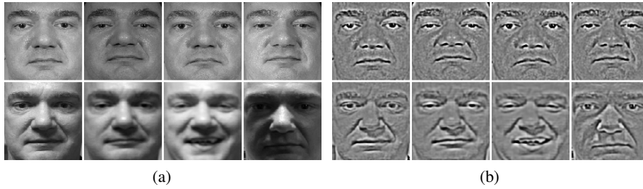
Fig. 3. Examples of images from FRGC-104: (a) target images (upper row) and query images (lower row) without illumination preprocessing; (b) the corresponding illumination normalized images from the proposed preprocessing chain.
