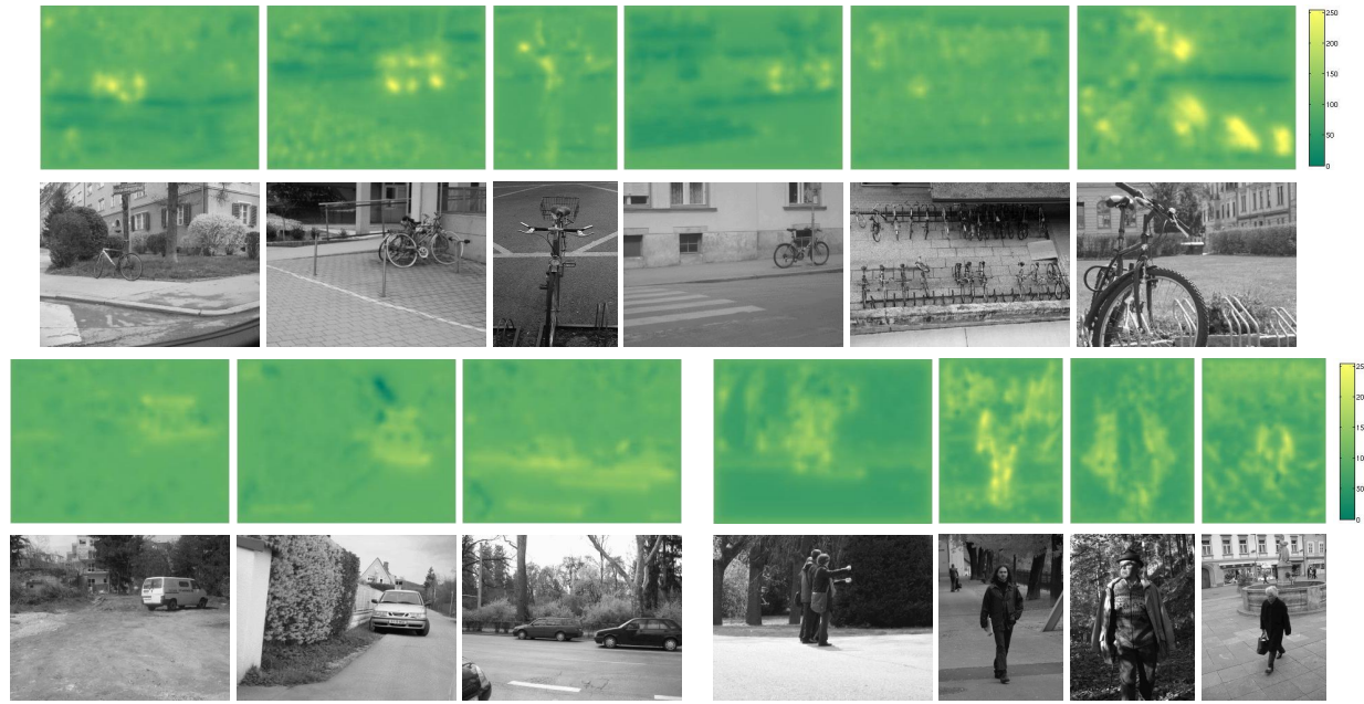
Figure 7. Pixelwise classification for a few example images (based on 4 \times 4 patches). (Top): Bikes, (Bottom Left): Cars, (Bottom Right): Persons. Dark green means a negative log likelihood (unlikely to be the object of interest); Light green and yellow indicate a positive log likelihood. Zero log likelihood corresponds to value 100 on the colorbar (best viewed in color).
