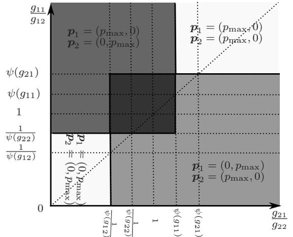
Fig. 2. Nash equilibrium action profiles as a function of the channel realization vector  $\mathbf{g} = (g_{11}, g_{12}, g_{21}, g_{22})$  for the two-player-two-channel game  $\mathcal{G}$ . Here, the function  $\psi : \mathbb{R}_+ \rightarrow \mathbb{R}_+$  is defined as follows:  $\psi(x) = 1 + \text{SNR}x$ . Note that it has been arbitrarily assumed that  $g_{21} > g_{11}$  and  $g_{12} > g_{22}$ .
