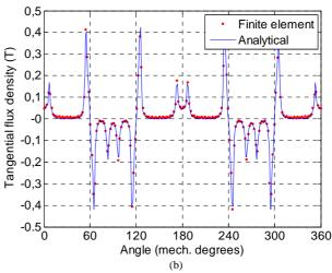
Fig. 8. Radial (a) and tangential (b) component of the flux density at no load in the middle of the airgap for  $\beta/\delta=0.4$
