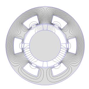
Fig. 13. Armature reaction magnetic flux distribution for  $J_{\it rms}\!\!=\!\!4.6A/\!mm^2$  and  $\beta/\delta=0.4$
