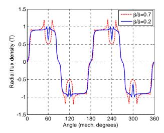
Fig. 9. Radial component of the flux density at no load in the middle of the airgap for  $\beta/\delta=0.2$  and  $\beta/\delta=0.7$ , analytical results.
