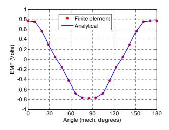
Fig. 10. Per turn phase back-EMF waveform for  $\beta/\delta = 0.4$  ( $\beta = 12^{\circ}$ )
