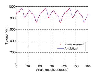
Fig.26. Electromagnetic torque versus rotor position for  $\beta/\delta$ =0.6 ( $J_{rms}$ =4.6A/mm<sup>2</sup>)
