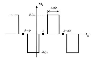
Fig. 6. Magnetization distribution along  $\theta$ -direction (PM rotor).
