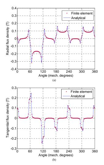
Fig. 14. Flux density distribution for radial (a) and tangential (b) component of armature reaction field in the middle of the airgap domain:  $J_{ms}$ =4.6 $A/mm^2$ ,  $I_a$ = I and  $I_b$  =  $I_c$  =-I/2, and  $\beta/\delta$  = 0.4.
