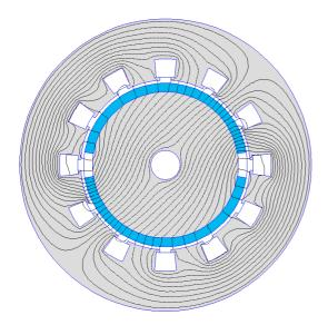
Fig. 24. Magnetic flux lines under load condition ( $\beta/\delta = 0.6$ )
