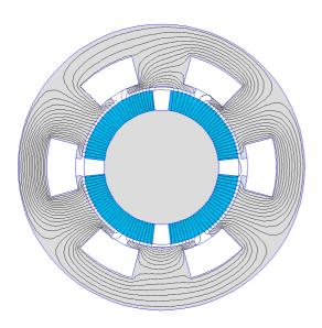
Fig. 17. Magnetic flux distribution for load condition ( $\beta/\delta = 0.4$ ).
