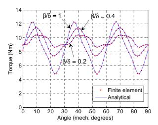
Fig. 20. Electromagnetic torque versus rotor position for different values of  $\beta/\delta$  ( $J_{rms}$ =4.6A/mm<sup>2</sup>)
