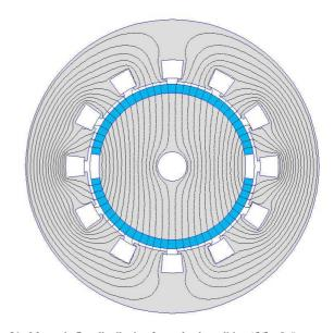
Fig. 21. Magnetic flux distribution for no-load condition ( $\beta/\delta = 0.6$ ).
