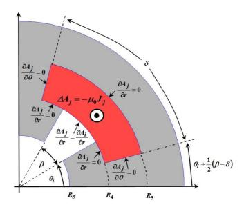
Fig. 3. jth slot subdomain with its boundary conditions (with homogeneous current density distribution  $J_i$  in the slot)
