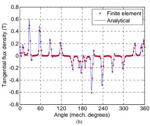
Fig. 25. Radial (a) and tangential (b) components of the airgap flux density under load conditions ( $\beta/\delta=0.6$ )
