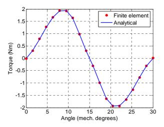
Fig. 11. Cogging torque waveform for  $\beta/\delta = 0.4$  ( $\beta = 12^{\circ}$ )
