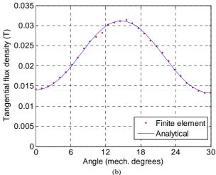
Fig. 16. Flux density distribution for radial (a) and tangential (b) component of armature reaction in the middle of the slot domain for  $\beta/\delta = 0.4$ .
