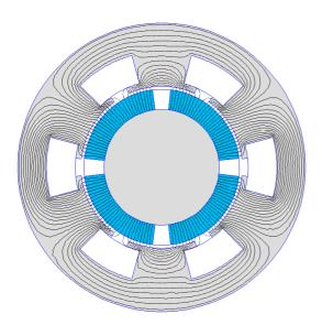
Fig. 7. Magnetic flux distribution for no-load condition ( $\beta/\delta = 0.4$ ).
