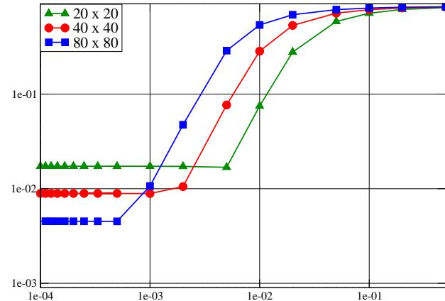
FIG. 6. Neumann case – Error for the pressure ( $L^\infty$ -norm) as a function of  $\delta t$ .
