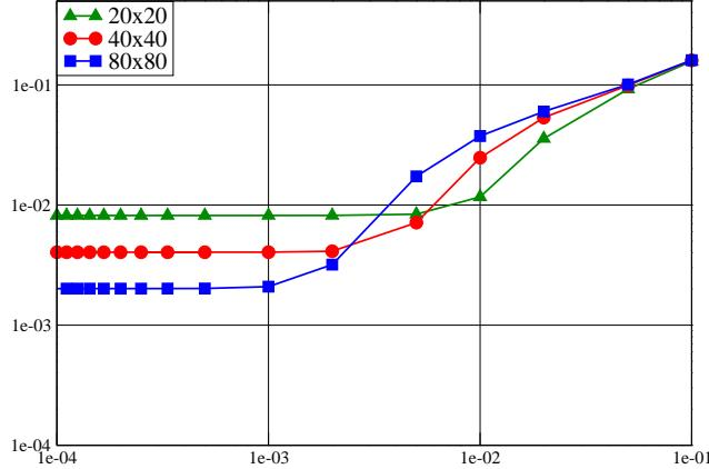
FIG. 5. Neumann case – Error for the pressure ( $L^2$ -norm) as a function of  $\delta t$ .
