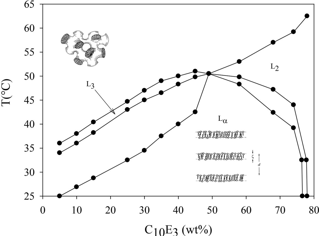
Figure1: Phase diagram of the C<sub>10</sub>E<sub>3</sub>-water system. The phases shown are the lamellar phase (L<sub>α</sub>), sponge phase
