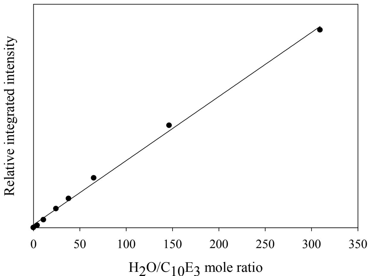
Figure 4: Relative integrated intensity of the O-H stretching band for the C<sub>10</sub>E<sub>3</sub>-water system after the subtraction of the contribution of the O-H stretching band of the surfactant, given as a function of the mole ratio of water to surfactant. The solid line shows the best linear fit passes through the origin.
