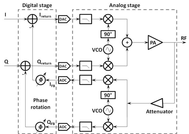
Figure 1. Zero-IF WCDMA transmitter with digital CFB loop
