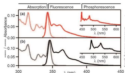
**Fig. 3** Absorption (dotted line) and fluorescence emission (solid line,  $\lambda_{\text{exc}} = 330$  nm) spectra of **1** (a) and **2** (b) in methylcyclohexane/2-methylpentane 1 : 1 at rt. Insets: phosphorescence spectra at 77 K.
