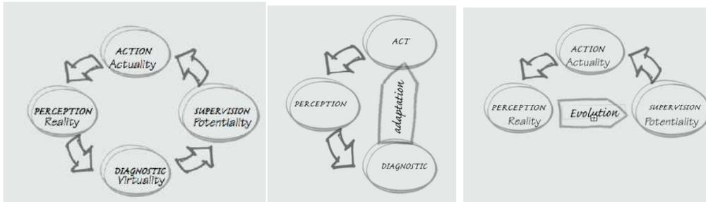
**Figures 1,2,3:** the Robot behaviour (fig1) is based on a causal temporal cycle producing an interpretation given by a sequence of actions. Brook Architecture (fig2) and the behavioral architecture (fig3) are based on more simple causal temporal cycle.
