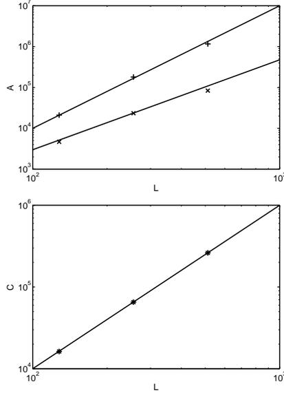
Fig. 3: Scaling of coefficients  $A$  (upper figure) and  $C$  (lower figure) defined in eq. (19). The straight lines are best fits and have slopes 3 for the  $\zeta = 0.8$  data (+) and 2.2 for the  $\zeta = 0.3$  data (x) in the upper figure. The theoretical values are 2.8 and 2.3 respectively. In the lower figure, the best fit has slope 2.0 for both the  $\zeta = 0.8$  and  $\zeta = 0.3$  data. The theoretical value is 2.
