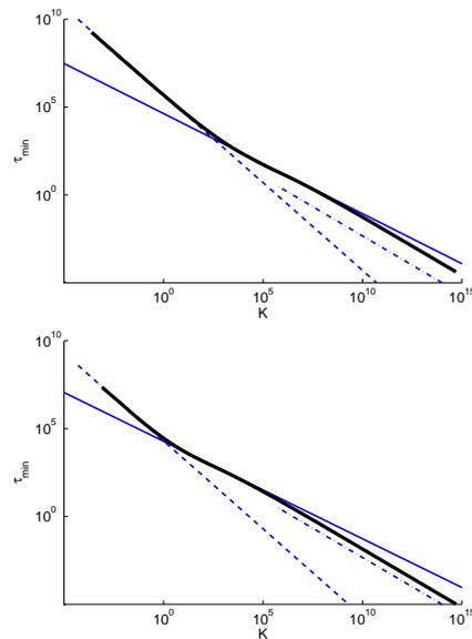
Fig. 4: First arrival time  $\tau_{\min}$  vs. permeability  $K$  for  $\zeta = 0.8$  (upper figure) and  $\zeta = 0.3$  (lower figure). Each curve is based on one sample of size  $512 \times 512$ . The slopes of the straight lines are given in the main text.
