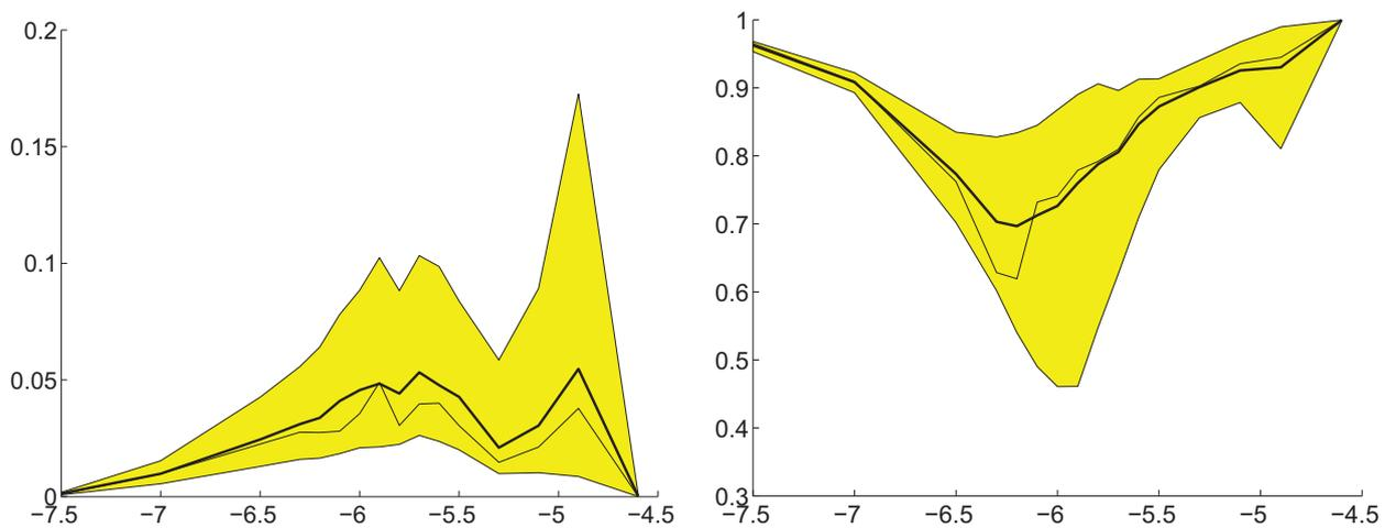
Figure 1. Confidence region of the random fraction function  $E_1^n(\eta)$  (left) and  $E_2^n(\eta)$  related to the random mechanical energy transferred to band  $B_1$  and  $B_2$ , respectively. Horizontal axis  $\log_{10} \eta$ . Vertical axis fraction in linear scale, adimensional.
