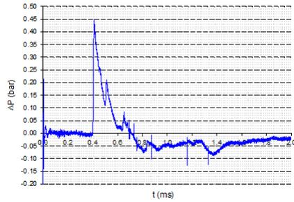
**Fig. 20** Pressure-time history - Sensor B - Wall 1 alone
