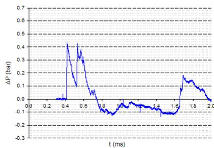
**Fig. 47** Time-evolution of pressure - Sensor C Walls 1 + 2 + 3
