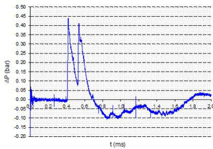
**Fig. 327** Pressure-time history - Sensor C - Wall 3
