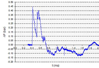
**Fig. 40** Pressure-time history - Sensor C - Walls 1 + 3
