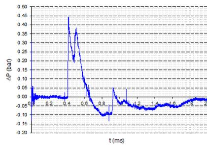
**Fig. 38** Pressure-time history - Sensor C - Wall 4
