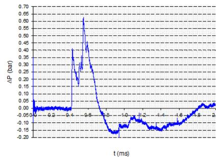
**Fig. 44** Pressure-time history - Sensor C - Walls 3 + 4
