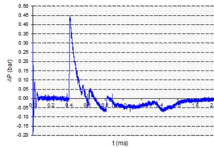
**Fig.23** Pressure-time history - Sensor B - Wall 4 alone
