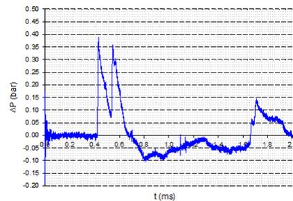
**Fig. 42** Pressure-time history - Sensor C - Walls 2 + 3
