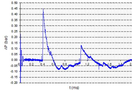
**Fig.21** Pressure-time history - Sensor B - Wall 2 alone
