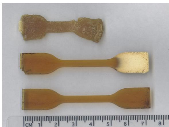
**Figure 13 - Photos of injection-molded N-5% samples from top to bottom: a) injection in cold mould for 30 s (25°C), b) injection in mould heated at 200°C for 30 s and left to cool down to 25°C for 6h. NB: the whitish left part of the sample is only an issue at the surface and cohesion is maintained in the bulk of the sample. c) injection in mould heated at 200°C for 30 s and water-cooled down to 25°C in 5 min.**
