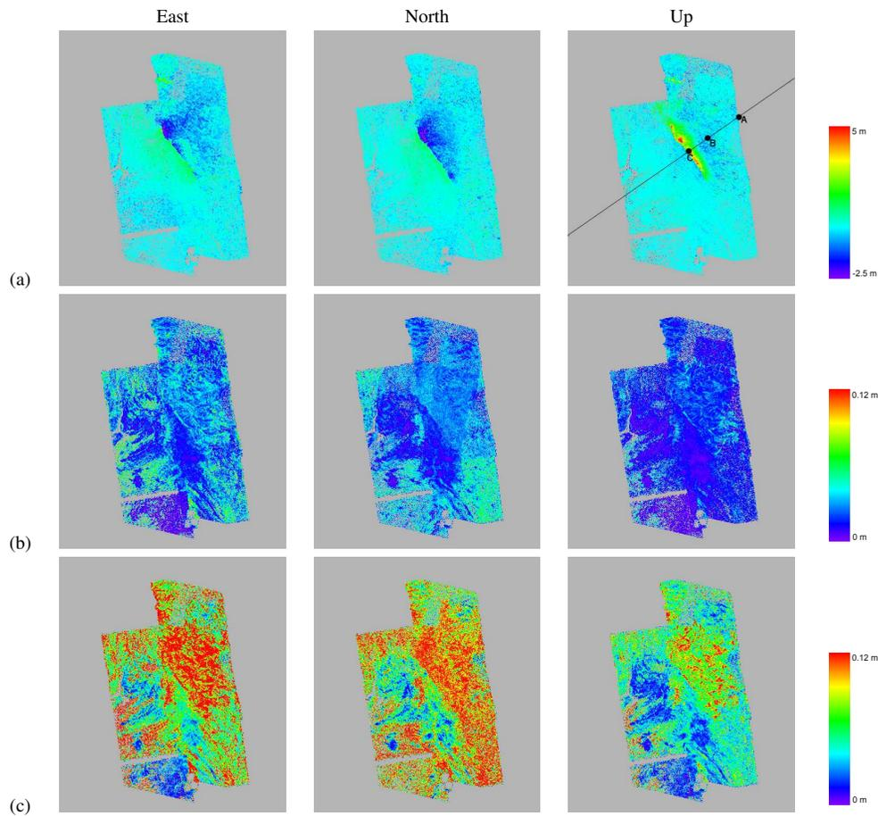
Fig. 3: (a) 3D displacement values (b) conventional uncertainty parameter values ( $\sigma$ ) (c) fuzzy uncertainty parameter values ( $h_{0.5}$ ) estimated in the linear case. The profile illustrated in (a) Up component, is used to compare the displacement values and uncertainties obtained in both linear and nonlinear case (Fig. 6). Point B and C are used for possibility distribution analysis (Fig. 5, Fig. 7).
