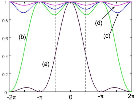
Fig. 7. One dimension (1D) angular response of the detection efficiency for the intensity  $\sum_m |\text{sinc}(X + m\pi)|^2$  as a function of  $X$  for the main lobe:  $m = 0$  (a); for the main lobe and 2 aliases:  $m = 0, \pm 1$  (b); for the main lobe and 4 aliases:  $m = 0, \pm 1, \pm 2$  (c); for the main lobe and 10 aliases:  $m = 0, \pm 1, \pm 2, \dots \pm 5$  (d).
