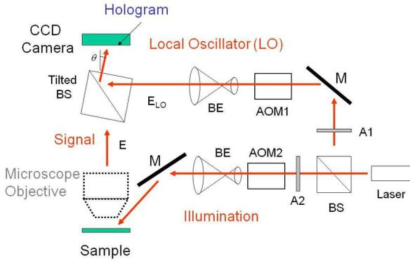
Fig. 1. Digital holography setup. AOM1 and AOM2 : acousto-optic modulators; BS : beam splitter; BE : beam expander; M : mirror; A1 and A2 : attenuator;  $\theta$  : tilt angle of the beam splitter with respect to optical axis
