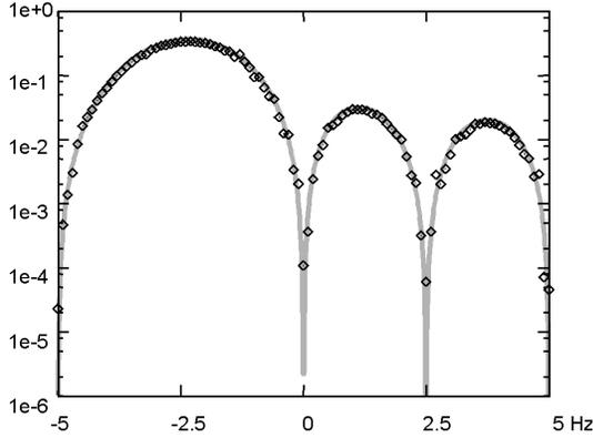
Fig. 4. Frequency response for heterodyne signal in intensity, as a function of the heterodyne beat frequency  $x = f - f_{LO}$  for a sequence of 4 frames: theory  $|\eta(x)|^2$  (heavy grey line), and experiment  $W(x)$  (points). Calculation and experiment are done with  $T = 0.1$  s. Vertical axis axis is  $|\eta(x)|^2$  or  $W(x)$  in logarithmic scales. Horizontal axis is  $x = f - f_{LO}$  in Hz.
