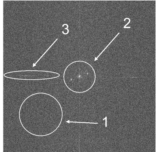
Fig. 6. Intensity image of  $\tilde{H}(k_x, k_y, 0)$  for  $4n = 4$  frames without signal  $\mathcal{E}$ . Three kind of noises can be identified. left : FFT aliasing, down left : shot noise, middle : technical noise of the CCD. By truncating the image and keeping only the left down part, the shot noise limit is reached. The image is displayed in arbitrary logarithm grey scale.
