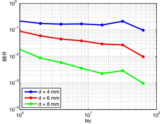
**Fig. 7.** Estimator performance with real 2D-BC through the estimation of  $p_{e|H_f}^d$  for 3 printing dimensions:  $d \in \{4, 6, 8\}$  mm. All 2D-BCs contain 1024 bits and were printed and scanned on a HP PhotoSmart C7200 (scan resolution: 1200dpi).
