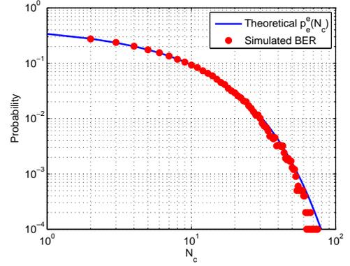
**Fig. 5.** Error probability of the estimator on the basis of theoretical equation (6) and evaluated with BER through simulations. Parameters:  $\alpha = 50$ ,  $\sigma_N^2 = 0, 3$ ,  $\Delta = 1$ ,  $S = 4$ .
