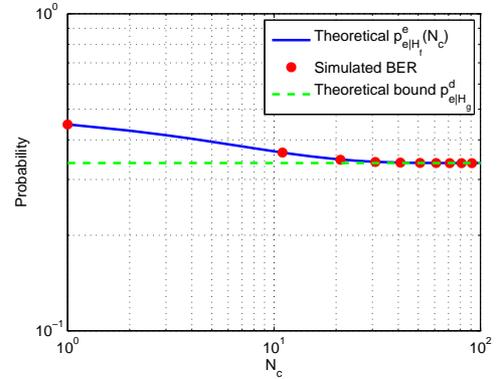
**Fig. 6.** Decoding error probability using fake contents on the basis of theoretical equation (8) and evaluated with BER through simulation, compared to the decoding error probability using genuine contents (equation (5)). Parameters:  $\alpha = 50$ ,  $\sigma_N^2 = 0, 3$ ,  $\Delta = 1$ ,  $S = 4$ .
