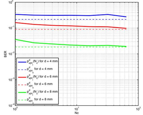
**Fig. 8.** Overall fake generation performance. When increasing  $N_c$ , Eve can ultimately reach Alice's decoder bound on authentic 2D-BCs (dashed lines): a fake can produce the same amount of errors as an authentic 2D-BC, which is good enough for Eve's goal.
