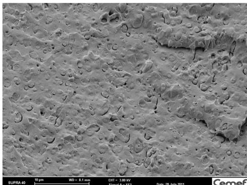
Fig. 1. SEM micrograph of a PLA/PHBV fractured sample with weight ratio 70/30.
