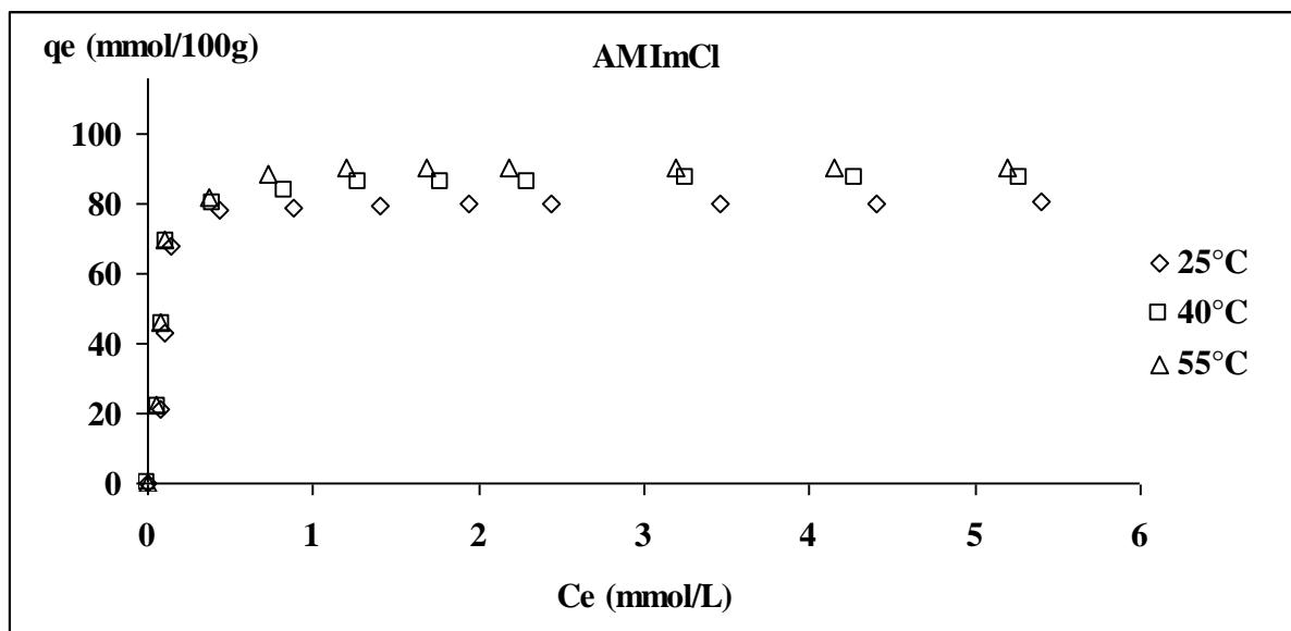
Figure 9 : experimental adsorption isotherms of AMImCl at  $25^\circ\text{C}$ ,  $40^\circ\text{C}$  and  $55^\circ\text{C}$ .
