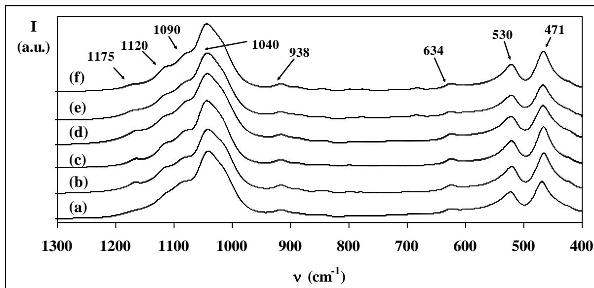
Figure 5 : FTIR spectra in the range  $400\text{-}1300\text{ cm}^{-1}$  of montmorillonite samples: raw (a), and after adsorption of BMImCl (b), OMImCl (c), AMImCl (d), BPyBr (e) and OPyBr (f).
