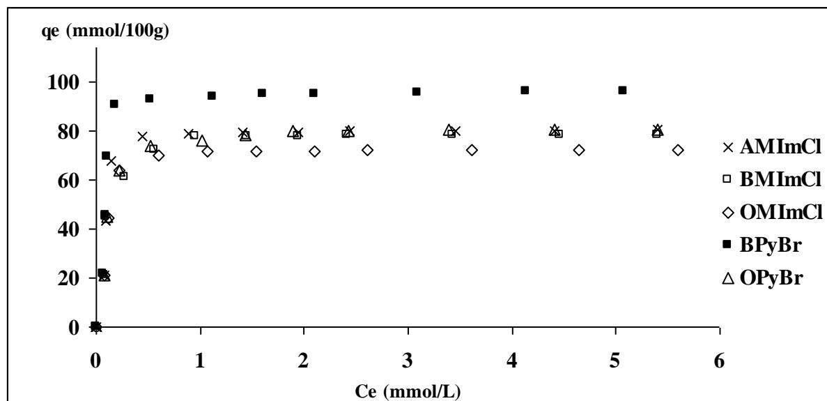
Figure 7 : adsorption isotherms of the five ionic liquids onto MMT at 25°C ([RTILs] = 0-7 mmol.L<sup>-1</sup>, m<sub>adsorbent</sub> = 0.05 g, V<sub>LI</sub> = 25 mL, contact time = 24 h)
