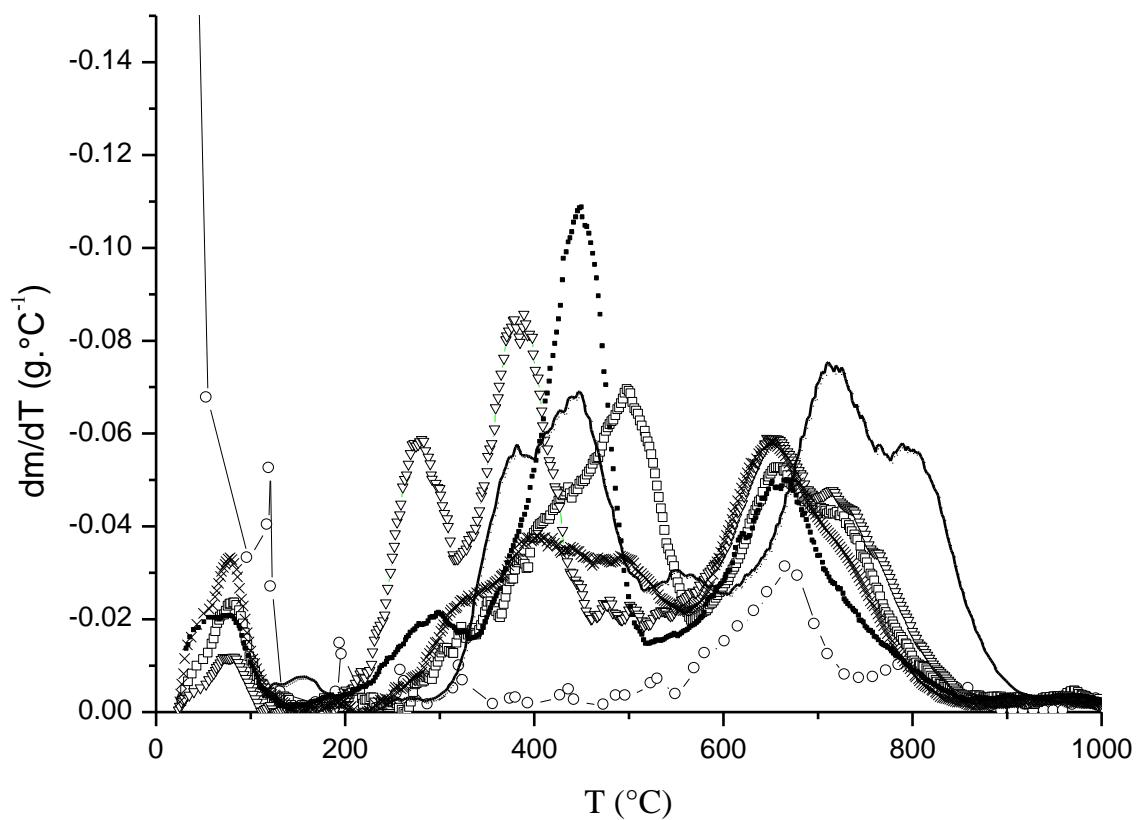
Figure 4 : DTG curves of montmorillonite samples : raw (O) and after adsorption of BMImCl (□), OMImCl (no symbol, full line), OPyBr (Δ), BPYBr (■) and AMImCl (×).
