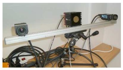
Fig. 4.2 A single ToF+2RGB system, as used in this chapter, with the ToF camera in the centre of the rail.
