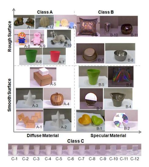
**Fig. 1.15** Test images categorized by their radiometric and geometric characteristics: Class A diffuse material objects (13 images), class B specular material objects (11 images) and class C translucent objects with subsurface scattering (12 images).
