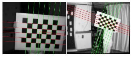
**Fig. 3.7** Example detections (cf. fig. 3.5) showing significant scale changes. The board on the right, which is in an image that shows background clutter and lens distortion, was not detected by OpenCV.
