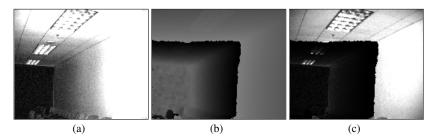
**Fig. 2.2** Amplitude correction example. (a) Amplitude image. (b) ToF depth map. (c) Corrected amplitude image. The intensity in (b) is proportional to the distance. The lower-left part of (b) has been wrapped. Images courtesy of Choi *et al.* [18].
