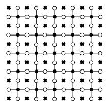
**Fig. 2.7** Graphical model that describes the zero-curl constraints (black discs) between neighboring shift variables (white discs). 3-element probability vectors ( $\mu$ 's) on the shifts between adjacent nodes (-1, 0, or 1) are propagated across the network. The x marks denote pixels [40].
