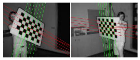
Fig. 3.5 Example detections in  $176 \times 144$  ToF amplitude images. The yellow dot (one-pixel radius) is the estimated centroid of the board, and the attached thick translucent lines are the estimated axes. The board on the right, which is relatively distant and slanted, was not detected by OpenCV.
