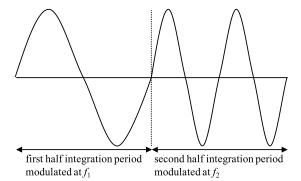
**Fig. 2.9** Frequency modulation within an integration period. The first half is modulated at  $f_1$ , and the other half is modulated at  $f_2$ .
