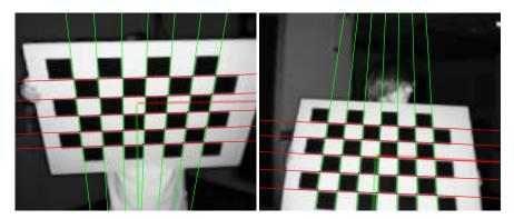
Fig. 3.6 Example detections (cf. fig. 3.5) showing significant perspective effects.
