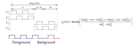
Fig. 1.8 Depth motion blur in 2-tap case.
