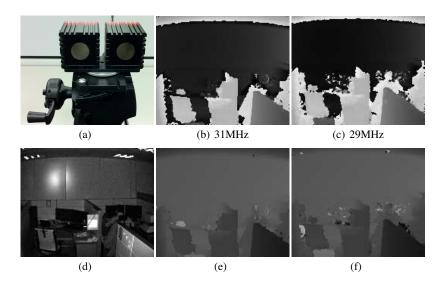
**Fig. 2.10** (a) Stereo ToF camera system. (b, c) Depth maps acquired by the system. (d) Amplitude image corresponding to (b). (e, f) Unwrapped depth maps, corresponding to (b) and (c), respectively. The intensity in (b, c, e, f) is proportional to the depth. The maximum intensity (255) in (b, c) and (e, f) correspond to 5.2m and 15.6m, respectively. Images courtesy of Choi and Lee [17].
