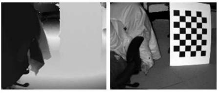
(b) IR Amplitude Error: 3D points of the same depth (chessboard on the left) show different IR amplitudes (chessboard on the right) according to the color of the target object.
