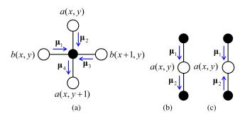
**Fig. 2.8** (a) Constraint-to-shift vectors are computed from incoming shift-to-constraint vectors. (b) Shift-to-constraint vectors are computed from incoming constraint-to-shift vectors. (c) Estimates of the marginal probabilities of the shifts given the data are computed by combining incoming constraint-to-shift vectors [40].
