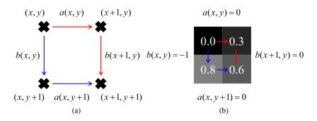
**Fig. 2.6** Zero-curl constraint: a(x,y) + b(x+1,y) = b(x,y) + a(x,y+1). (a) The number of relative wrappings between (x+1,y+1) and (x,y) should be consistent regardless of its integrating paths. For example, two different paths (red and blue) are shown. (b) shows an example in which the constraint is not satisfied. The four pixels correspond to the four pixels in the middle of fig. 2.5(a).
