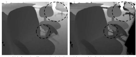
(a) Light Scattering: IR saturation in the lower-right part of the depth image causes depth distortion in other parts, as indicated by dashed circles.
