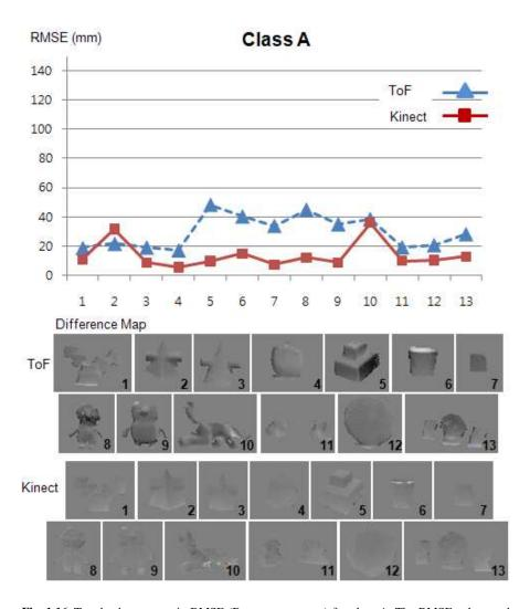
**Fig. 1.16** ToF depth accuracy in RMSE (Root mean square) for class A. The RMSE values and their corresponding difference maps are illustrated. 128 in difference map represents zero difference while 129 represents the ground truth is 1 mm larger than the measurement. Likewise, 127 indicates that the ground truth is 1 mm smaller than the measurement.
