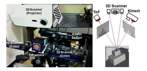
Fig. 1.12 Heterogeneous camera setup for depth sensing.
