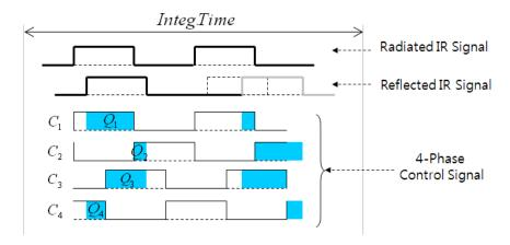
**Fig. 1.2** Depth can be calculated by measuring the phase delay between radiated and reflected IR signals. The quantities  $Q_1$  to  $Q_4$  represent the amount of electric charge for control signals  $C_1$  to  $C_4$  respectively.
