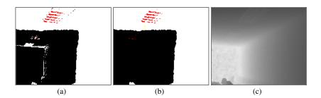
Fig. 2.3 Detection of wrapped regions. (a) Result obtained by expectation maximization. (b) Result obtained by MRF optimization. The pixels with labels L and H are colored in black and white, respectively. The red pixels are those with extremely high or low amplitude values, which are not processed during the classification. (c) Unwrapped depth map corresponding to fig. 2.2(b). The intensity is proportional to the distance. Images courtesy of Choi *et al.* [18].
