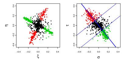
**Fig. 3.2** Left: the cruciform distribution of image gradients, due to black/white and white/black transitions at each orientation, would be difficult to segment in terms of horizontal and vertical components  $(\xi, \eta)$ . Right: the same distribution is easily segmented, by eigen-analysis, in the double-angle representation (3.7). The red and green labels are applied to the corresponding points in the original distribution, on the left.
