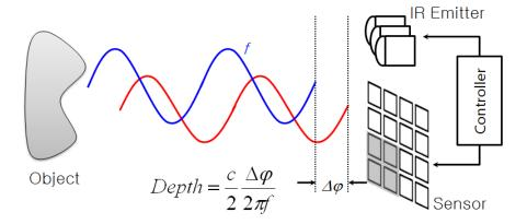
Fig. 1.1 The principle of ToF depth camera [37, 71, 67]: The phase delay between emitted and reflected IR signals are measured to calculate the distance from each sensor pixel to target objects.
