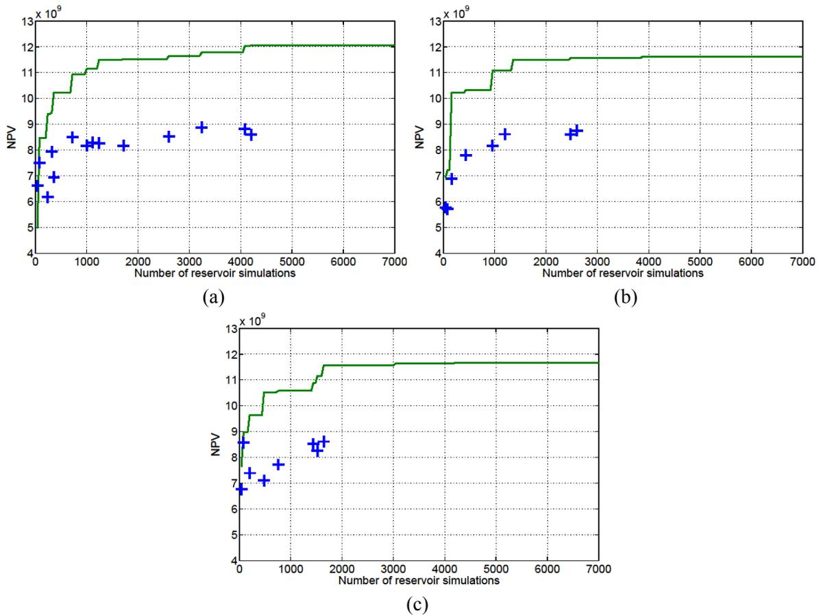
**Figure 8** The evolution of the well placement optimization process on the PUNQ-S3 case using CMA-ES with the “using one realization” approach, for three independent runs in (a), (b) and (c). The evolutions of the best estimated objective function (equal to an evaluation on a randomly chosen realization) are drawn with green lines. The evaluations on the true objective function over the 20 possible realizations, i.e.,  $NPV^R$  are depicted with blue crosses.
