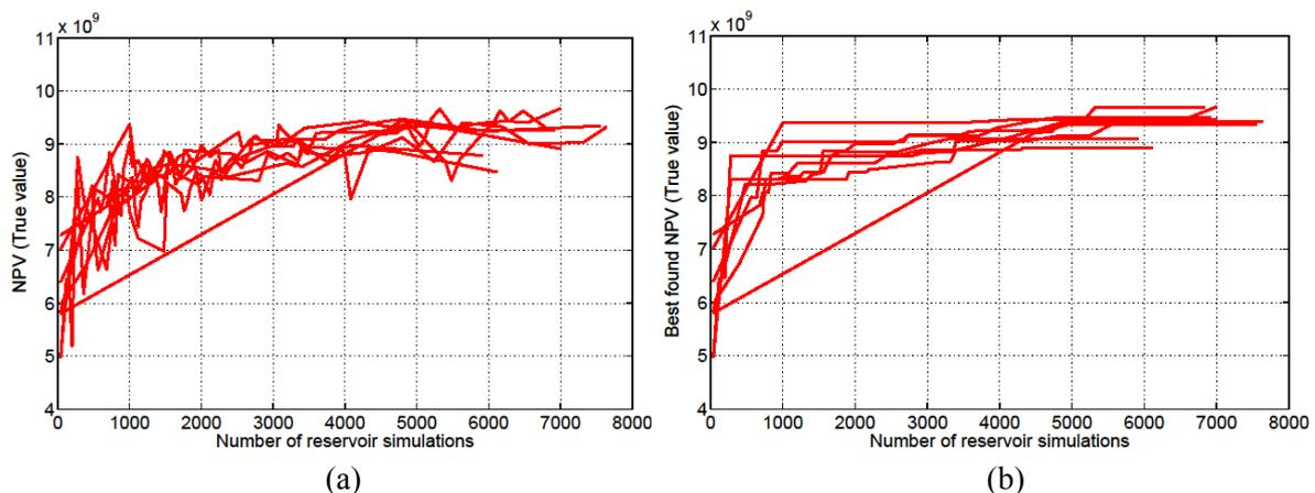
**Figure 4** The evolution of the well placement optimization process on the PUNQ-S3 case using CMA-ES with the “using the neighborhood” approach for eight independent runs. (a) shows the evolution of the evaluations on  $NPV^R$ . (b) shows the evolution of the best found evaluation on  $NPV^R$ . The maximum distance of selection for the neighborhood  $d_{max}$  is equal to 4000.
