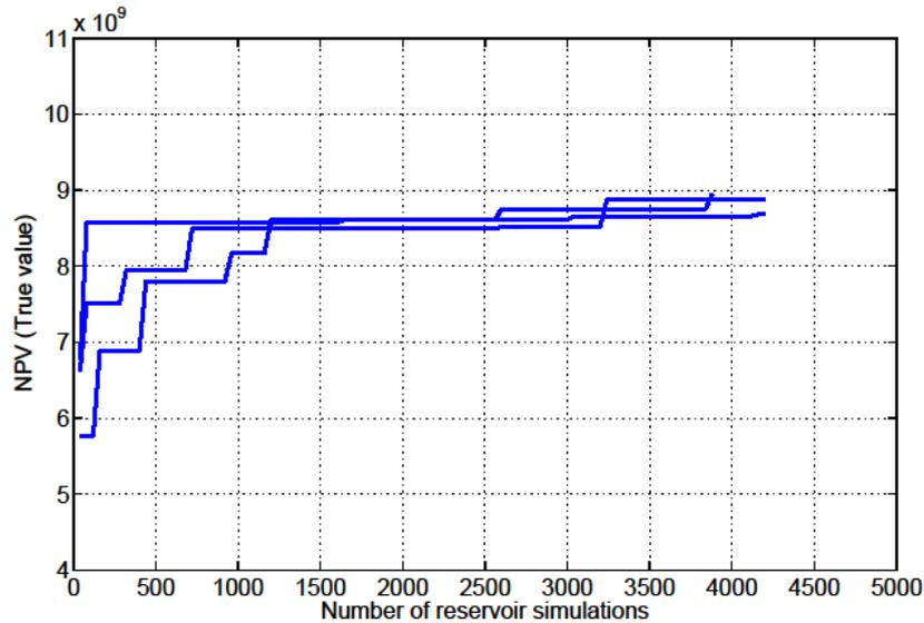
**Figure 9** The evolution of the well placement optimization process on the PUNQ-S3 case using CMA-ES with the “using one realization” approach. The best mean value of the NPV over the 20 possible realizations, i.e.,  $NPV^R$  is shown. Three runs are performed.
