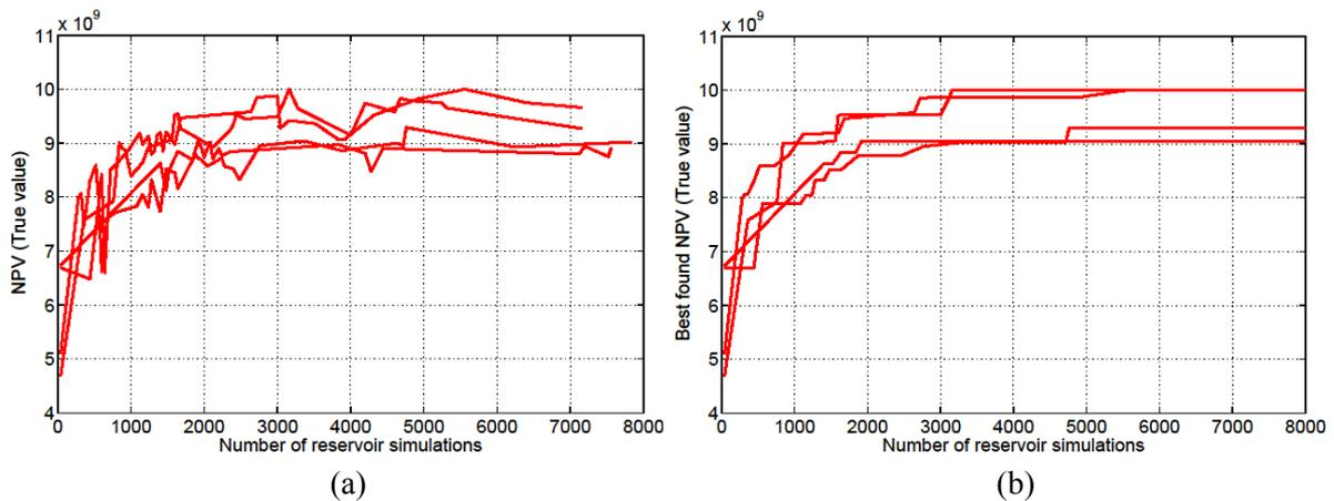
**Figure 6** The evolution of the well placement optimization process on the PUNQ-S3 case using CMA-ES with the “using the neighborhood” approach for four independent runs. (a) shows the evolution of the evaluations on NPV<sup>R</sup>. (b) shows the evolution of the best found evaluation on NPV<sup>R</sup>. The maximum distance of selection for the neighborhood  $d_{\max}$  is equal to 3000.
