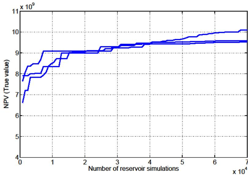
**Figure 2** The evolution of the well placement optimization process on the PUNQ-S3 case using CMA-ES with the “using the mean of samples” approach. The best mean value of the NPV over the 20 possible realizations, i.e.,  $NPV^R$  is shown. Three runs are performed.
