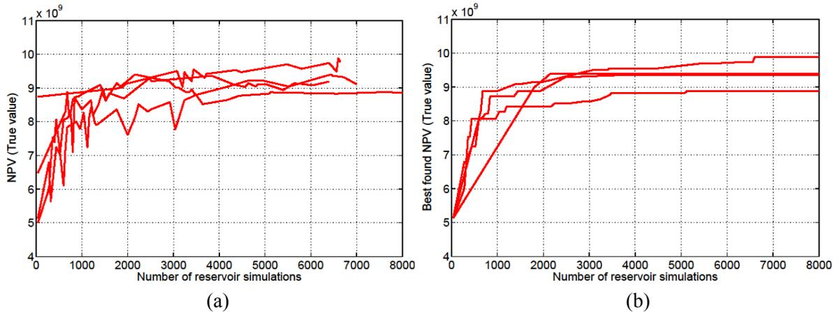
**Figure 7** The evolution of the well placement optimization process on the PUNQ-S3 case using CMA-ES with the “using the neighborhood” approach for four independent runs. (a) shows the evolution of the evaluations on  $NPV^R$ . (b) shows the evolution of the best found evaluation on  $NPV^R$ . The maximum distance of selection for the neighborhood  $d_{max}$  is equal to 6000.
