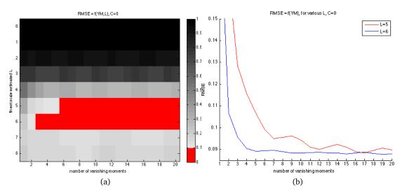
Figure 4: RMSE between estimated  $\hat{v}$  and reference motion  $v_{ref}$  as a function of the number of vanishing moments (VM) and the finest scale *L*, with *C* = 0 here. Region of interest, with RMSE < 0.1 pixel, is colored in *red*. It corresponds to *L* = 5; 6. Fig. (4b) plots slices from Fig. (4a) taken at *L* = 5 (*red*) and 6 (*blue*).
