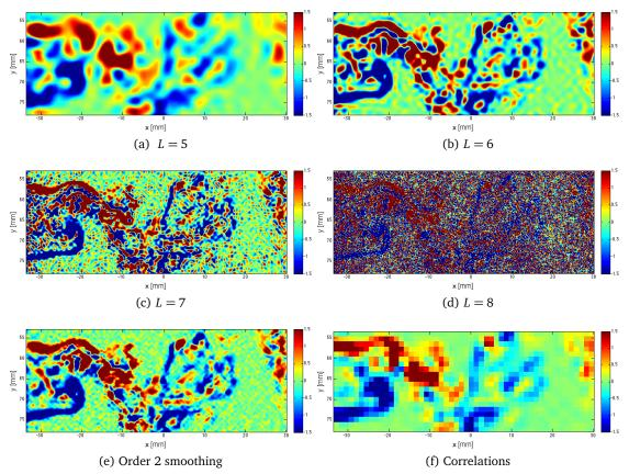
Figure 11: Vorticity comparison. Estimates (11a), (11b), (11c), (11d) are obtained with proposed estimator, varying parameter L. Motion (11e) is obtained with a more evolved estimator featuring explicit smoothing terms [10]. Last estimate (11f) is a reference given by the correlation-based method.
