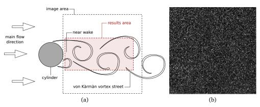
Figure 10: Configuration of the cylinder wake experiment (10a); a  $256 \times 256$  pixels subregion (1/16 of the total area) of a sample of PIV image (10b).
