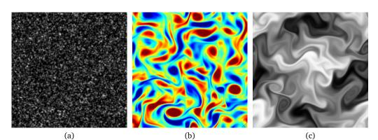
Figure 3: The first frame of the synthetic *PIV image* sequence (3a) with the *vorticity* of the underlying reference velocity field  $v_{ref}$  (3b). A sample frame from the synthetic *passive* scalar advection-diffusion sequence (3c).
