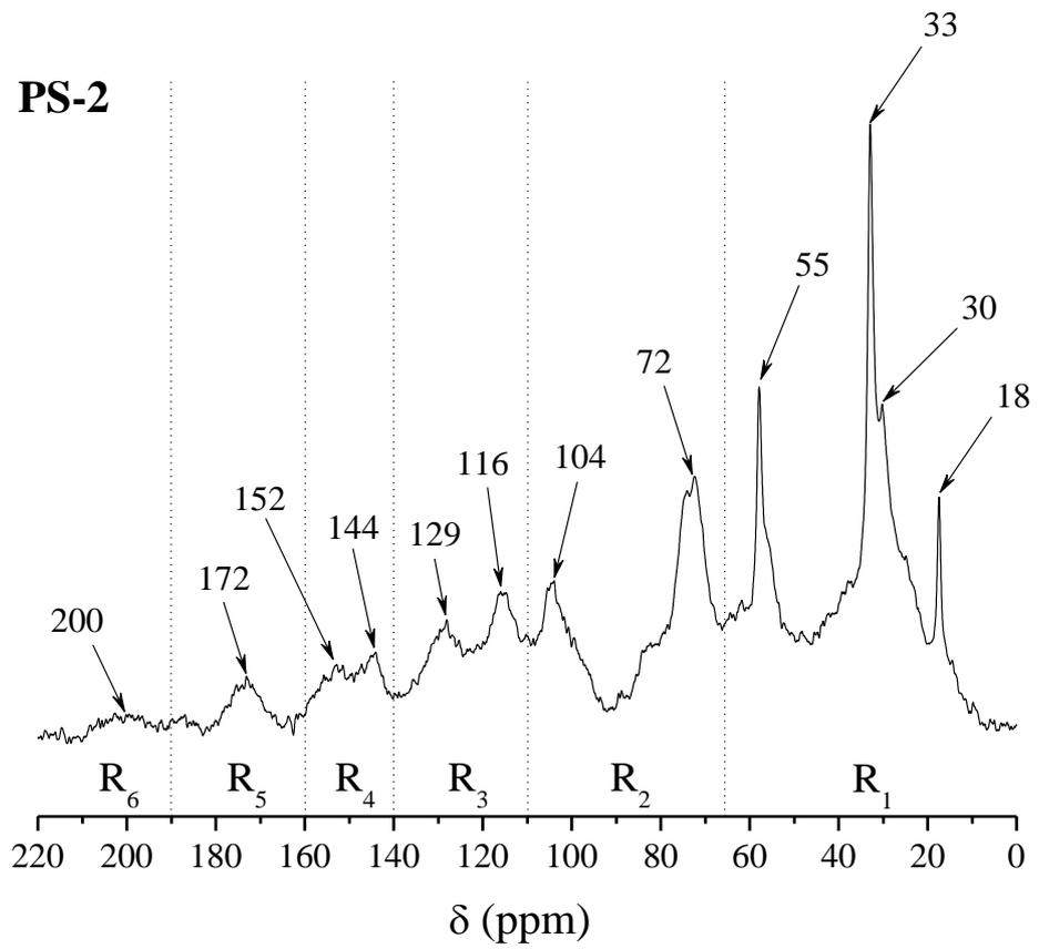
**Fig. 7** Solid-state  $^{13}\text{C}$  NMR spectra of the peat samples.
