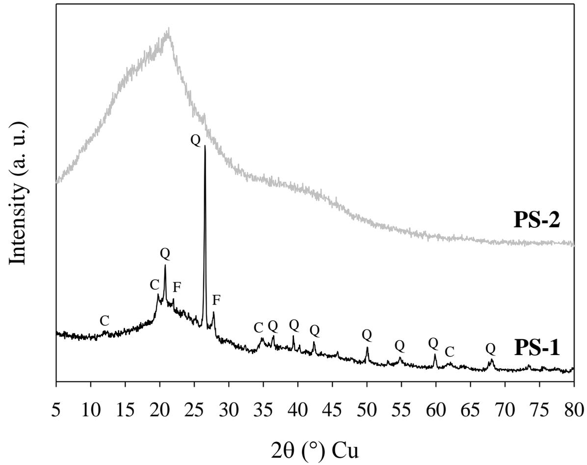
**Fig. 5** XRD diffractograms of the peat samples (where C = clay, F = feldspar; Q = quartz).
