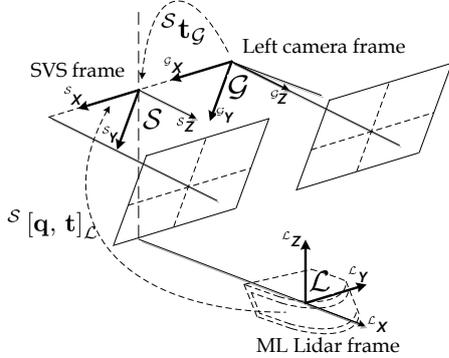
**Fig. 5** The multi-sensor frames are located at the optical center of the left camera,  $\mathcal{G}$ , the midpoint of the SVS,  $\mathcal{S}$ , and the ML-lidar sensor,  $\mathcal{L}$ .
