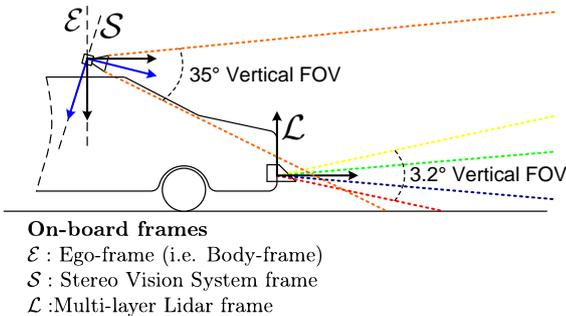
**Fig. 6** On-board frames and exteroceptive vertical sensor coverage. The depicted lidar layer divergence and the camera FOV have been exaggerated for clarity.
