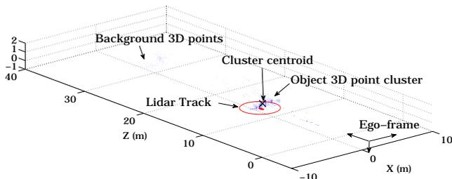
Fig. 20 3D visualization of a confirmed track using 3D point clusters
