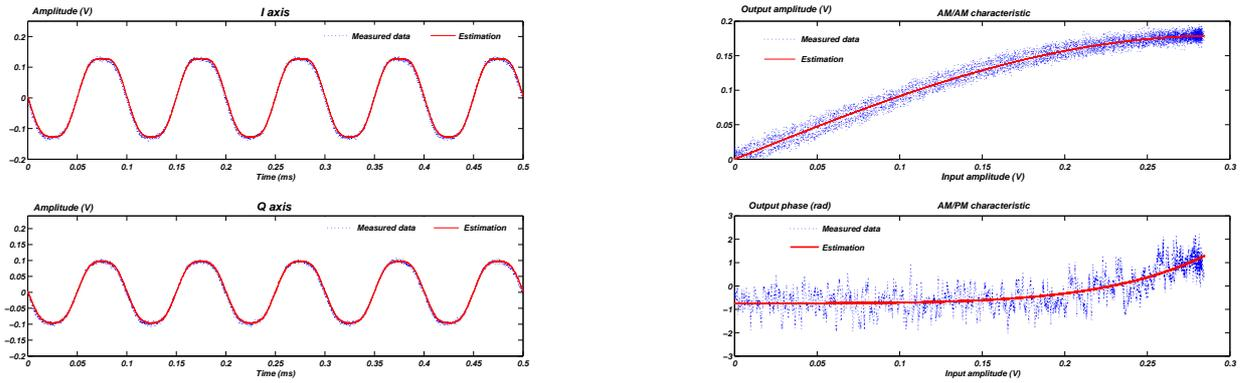
Fig. 4. (a) Comparison of time-domain measurement and estimation for sinusoidal input (b) Comparison between the measured and estimated AM/AM and AM/PM functions
