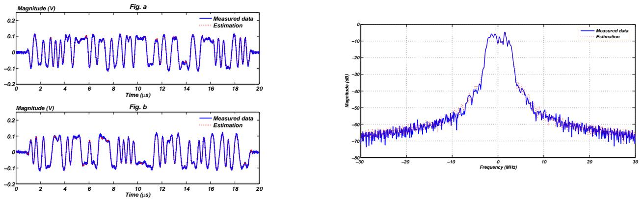
Fig. 7. (a) Time-domain measurement and estimation for QPSK modulation (b) Measured and estimated output spectrum
