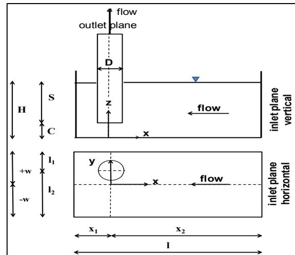
Figure 1. Pump-sump shape and geometrical
