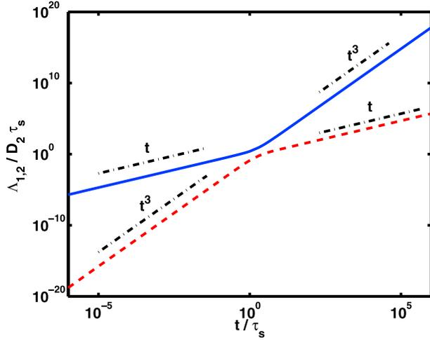
**Figure 3.** Spatial variance along the main axes of the variance tensor for  $D_1 = 0$  in equation (8). The behavior of  $\Lambda_1(t)$  is shown by the solid blue line, while the behavior of  $\Lambda_2(t)$  is shown by the dashed red line. The dash-dotted black lines illustrate slopes of  $t$  and  $t^3$ .
