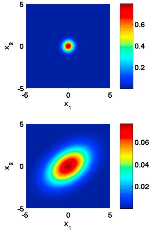
**Figure 2.** Concentration fields for  $D_1 = 1$ ,  $D_2 = 1$ ,  $\alpha = 1$  at (top)  $t = 0.1 \tau_s$  and (bottom)  $t = 10 \tau_s$ . The initial condition is a point-like distribution at the origin, and the mean flow is  $q = 0$ .
