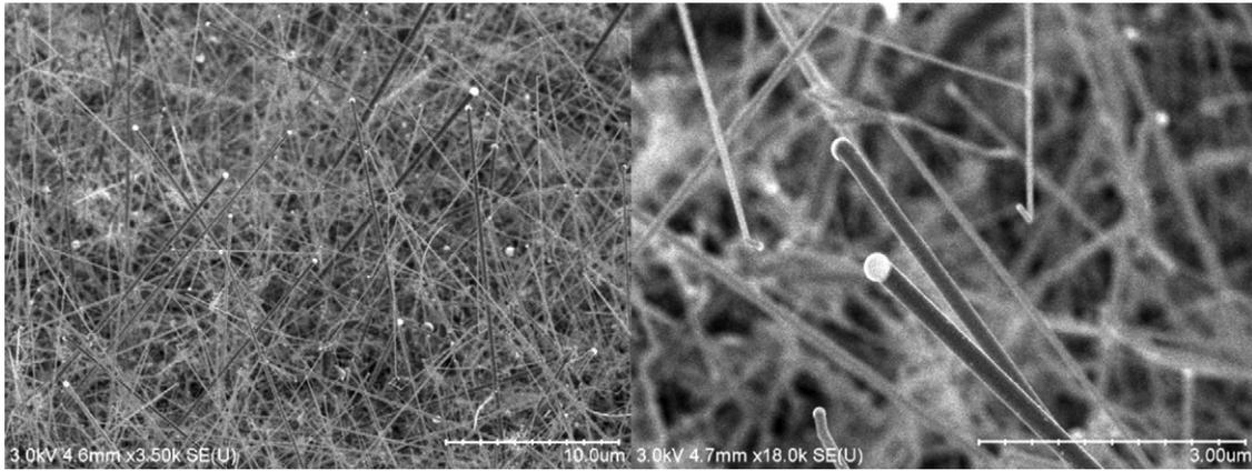
Fig. 2. SEM observations of SiNWs films obtained at 550 °C.
