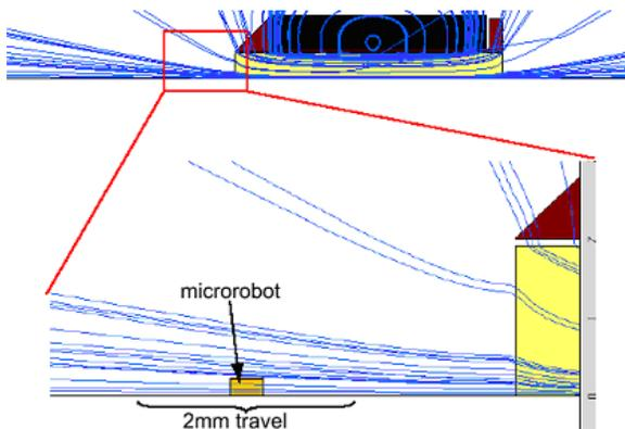
Fig.9 Streamline of the magnetic field.
