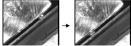
Fig.1 Early experiments on a  $500 \times 500 \times 200 \mu\text{m}^3$  piece of PMN-PT material validated sliding conditions upon applying step impulses of (0...+300)V at 100 Hz. The frames are taken at  $\sim 100\text{ms}$  interval.
