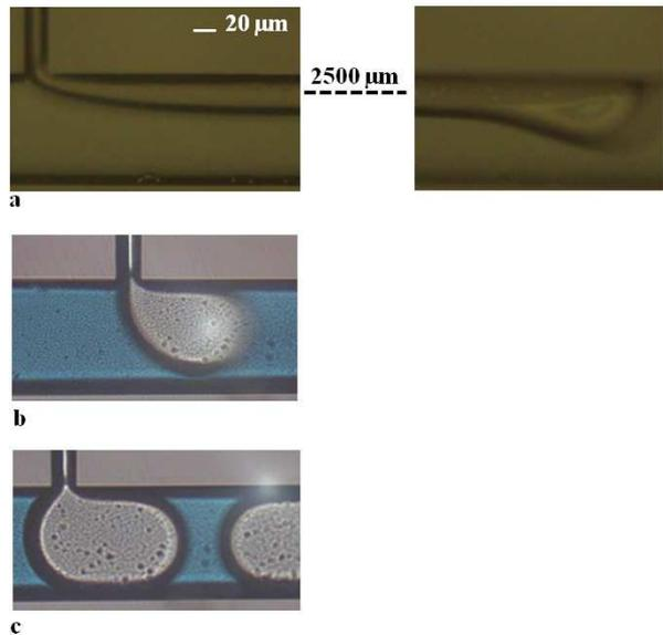
**Fig. 1** View of the jetting regime (a), the dripping regime (b) and the squeezing regime (c), with  $w_c = 100 \mu\text{m}$ ,  $w_d = 20 \mu\text{m}$ ,  $\bar{v}_d = 20 \text{ mm/s}$  and  $\bar{v}_c = 50 \text{ mm/s}$  (a),  $\bar{v}_d = 12 \text{ mm/s}$  and  $\bar{v}_c = 14 \text{ mm/s}$  (b),  $\bar{v}_d = 12 \text{ mm/s}$  and  $\bar{v}_c = 2.3 \text{ mm/s}$  (c).
