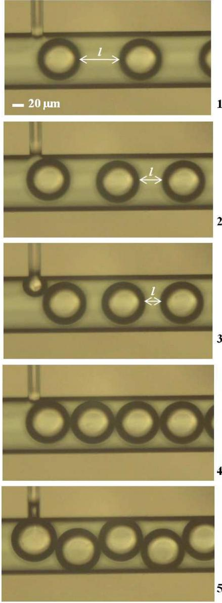
**Fig. 7** Distance between two consecutive droplets with  $w_c = 100 \mu\text{m}$ ,  $w_d = 20 \mu\text{m}$ ,  $\bar{v}_d = 2.1 \text{ mm/s}$  and  $\bar{v}_c = 1.2 \text{ mm/s}$  (1),  $1 \text{ mm/s}$  (2),  $0.85 \text{ mm/s}$  (3),  $0.65 \text{ mm/s}$  (4) and  $0.62 \text{ mm/s}$  (5).
