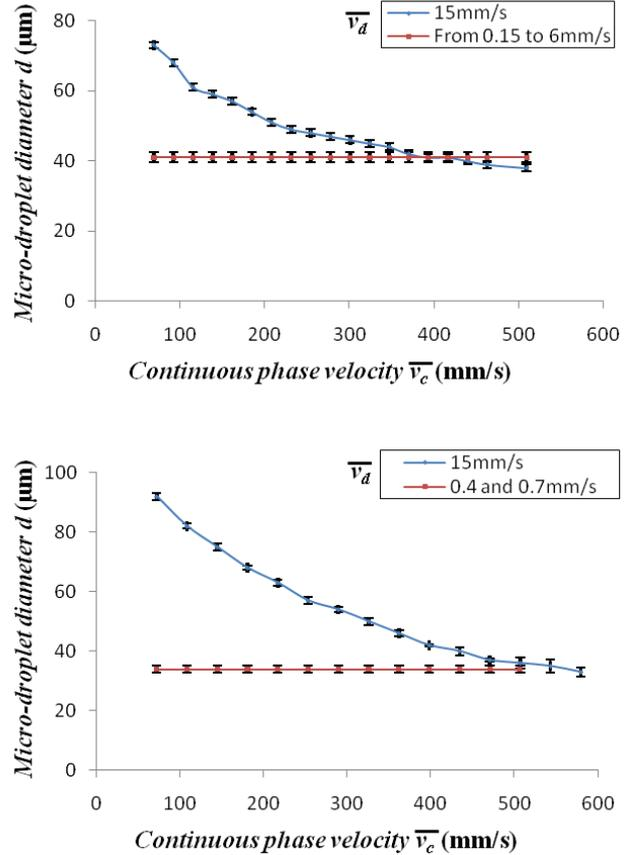
**Fig. 6** Effect of the continuous phase velocity on the micro-droplet diameter in the dripping regime (Tarchichi et al 2012) and the new regime with  $w_c = 100$   $\mu$ m,  $w_d = 10$   $\mu$ m and  $h = 72$  (a), 46 (b).
