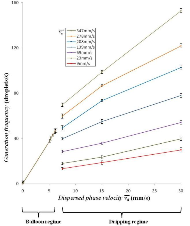
**Fig. 8** Effect of the dispersed phase velocity on the frequency of the micro-droplet generation for different values of the continuous phase velocity with  $w_c = 100 \mu\text{m}$ ,  $w_d = 10 \mu\text{m}$  and  $h = 72 \mu\text{m}$ .
