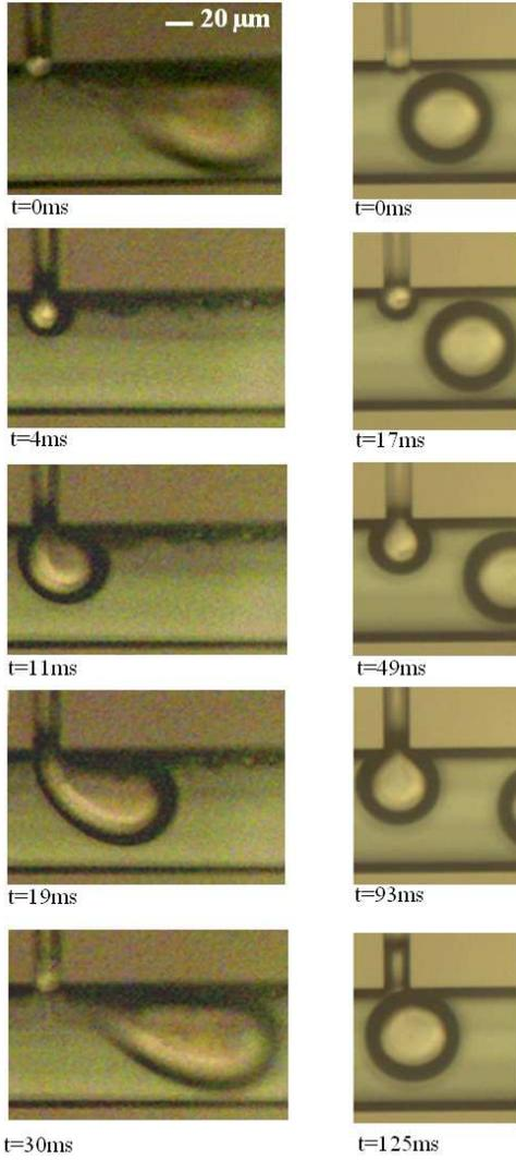
**Fig. 4** Comparison between the process of the droplet formation in the dripping regime (left) for  $\bar{v}_d = 15$  mm/s,  $\bar{v}_c = 72.5$  mm/s (Tarchichi et al 2012), and the balloon regime (right) for  $\bar{v}_d = 2.1$  mm/s,  $\bar{v}_c = 1.2$  mm/s ( $w_d = 20$   $\mu$ m,  $w_c = 100$   $\mu$ m and  $h = 46$   $\mu$ m).
