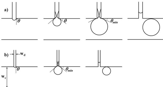
**Fig. 5** Schematic of the micro-droplet detachment in the balloon regime with  $w_c = 100$   $\mu$ m and  $w_d = 20$   $\mu$ m (a), and 10  $\mu$ m (b).
