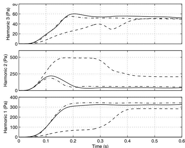
Figure 5: Amplitude of the three first harmonics versus time during a fast attack for one amplitude of coupling ( $p/p_{ac} = 0.6$ ) for phases: (solid line) reference signal without coupling, (dashed line)  $\varphi = \pi$ , (dot-dashed line)  $\varphi = -\pi/4$ . The main differences occur for a phase coupling close to  $\pi$ .
