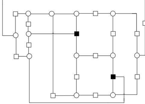
Figure 3.3: (12, 2) Stopping set present in graph of the (732, 551)  $d_{min} = 12$  code
