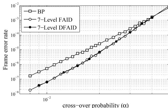
Figure 3.2: Frame error rate performance comparison of Belief Propagation (BP), Finite Alphabet Iterative Decoder (FAID), and Decimation-enhanced FAID (DFAID) on the (155, 64) Tanner code
