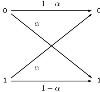
Figure 1.1: Illustration of the Binary Symmetric channel
