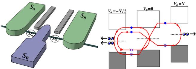
FIG. 1: (color online) A Josephson bijunction (left). Superconductors  $S_\alpha$  ( $\alpha = a, b$ ) are biased at voltages  $V_\alpha$ , while  $S_0$  is grounded. The distance between the two quantum dot junctions is comparable to the coherence length. The right panel shows the energy diagram for the  $S_a D_a S_0 D_b S_b$  bijunction and a higher order diagram associated with a “sextet” current with 3 pairs emitted, 2 in  $S_a$  and 1 in  $S_b$ , with  $V_a = -V_b/2$ .
