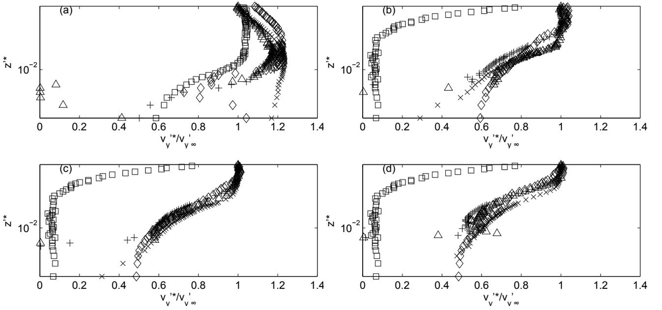
Fig. 15. Longitudinal non-dimensional velocity profile  $v'_y/v'_{y\infty}$  of the non-cavitating flow, at (a)  $y^* = 0$ , (b)  $y^* = 0.5$ , (c)  $y^* = 1$  and (d)  $y^* = 2$ .  $\times$ : plate 0,  $\diamond$ : plate 2,  $+$ : plate 6,  $\diamond$ : plate 7,  $\square$ : plate 8.
