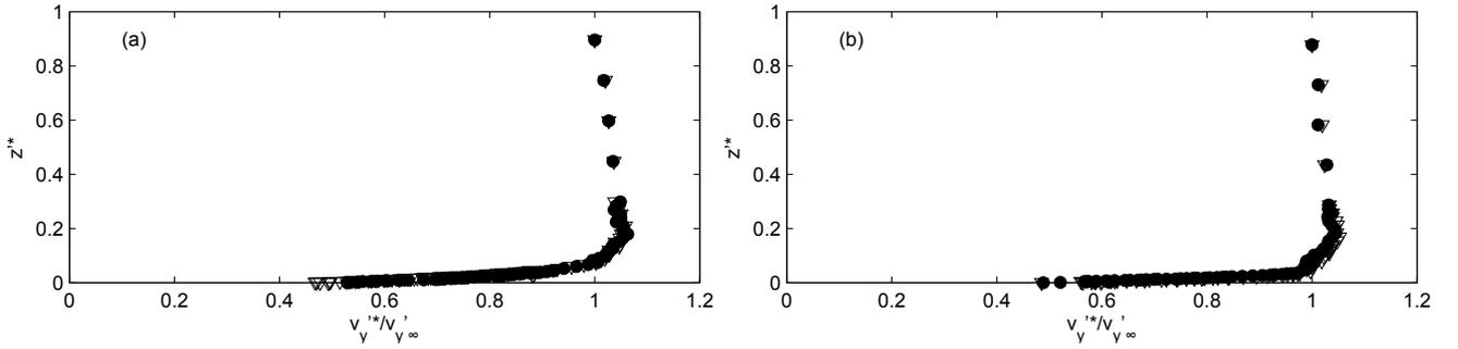
Fig. 16. Longitudinal non-dimensional velocity profile  $v_y'^*/v_{y\infty}'$  of the non-cavitating flow, at  $y^* = 0.5$ , for (a) the grooved sheet 6 and (b) the grooved sheet 2.  $\bullet$ :  $x^* = 0$ ,  $\triangle$ :  $x^* = \frac{\lambda}{2}$
