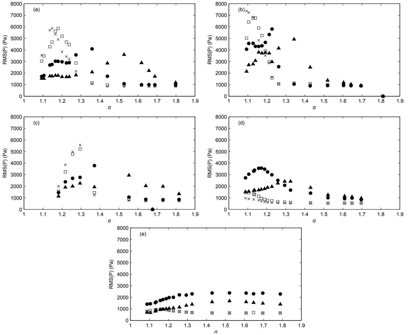
Fig. 9. Pressure fluctuations  $RMS(P)$  on the Venturi bottom wall according to the cavitation number  $\sigma$ , at different distances from the ventrui throat:(a) for plate 0,(b) for plate 2, (c) for plate 6, (d) for plate 7 and (e) for plate 8.  $\blacktriangle$ : C1,  $\bullet$ : C2,  $\square$ : C4,  $\times$ : C6. (see positions of sensors in Table 2)
