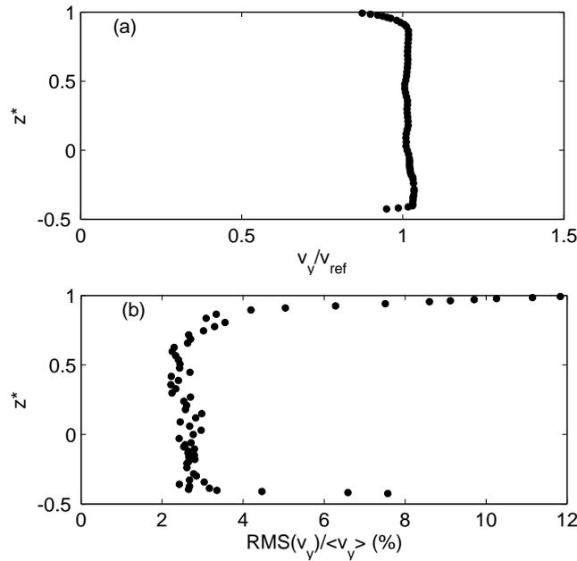
Fig. 2. Characterisation of the flow in the test section inlet: (a) undimensional longitudinal velocity profile  $v_y^* = v_y / v_{ref}$  (the line represents the mean value of the velocity  $v_{ref} = 5.56 \text{ m}\cdot\text{s}^{-1}$ ) and (b) the profile of the turbulence intensity  $\frac{RMS(v_y)}{\langle v_y \rangle}$ , where  $\langle v_y \rangle$  is the time-averaged velocity,  $y^* \simeq -4.5$  and  $x^* = 0$  (Results come from LDV measurements, presented in the section 4.1).
