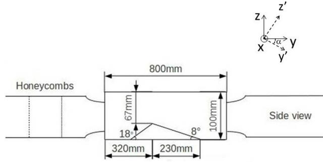
Fig. 1. Test section of the experimental device using a Venturi profile (the origin of the cartesian coordinate system is located at the throat, in the middle of the test section wide,  $\alpha = 8^\circ$  is the angle for the LDV measurements system  $xy'z'$  and  $H_{throat} = 67$  mm is the reference length).
