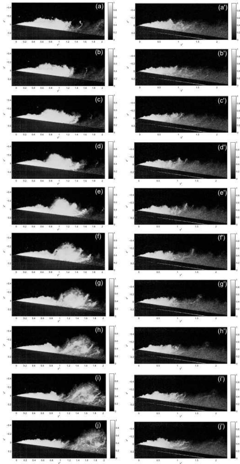
Fig. 14. Visualisation of (a-j) the cloud cavitation shedding for the smooth plate 0 and (a'-j') the sheet cavity pulsation for the plate 8, when  $\sigma = 1.17$  ( $\Delta t = 2$  ms between two images)
