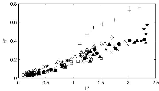
Fig. 7. Undimensional sheet cavity mean height  $H^* = H/H_{throat}$  according to the undimensional sheet cavity mean length  $L^* = L/H_{throat}$ :  $\times$ : plate 0,  $\star$ : plate 1,  $\triangle$ : plate 2,  $\blacktriangle$ : plate 3,  $+$ : plate 4,  $\star$ : plate 5,  $+$ : plate 6,  $\diamond$ : plate 7,  $\square$ : plate 8.
