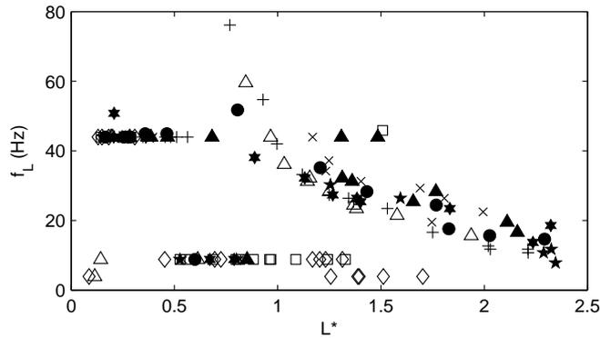
Fig. 10. Frequency of the sheet cavity length oscillation  $f_L$  according to the undimensional sheet cavity mean length  $L^*$ :  $\times$ : plate 0,  $\star$ : plate 1,  $\triangle$ : plate 2,  $\ast$ : plate 3,  $+$ : plate 4,  $\star$ : plate 5,  $+$ : plate 6,  $\diamond$ : plate 7,  $\square$ : plate 8.
