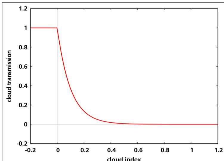
Figure 7.7. Example of transfer function from cloud observation (cloud index) to cloud transmission.
