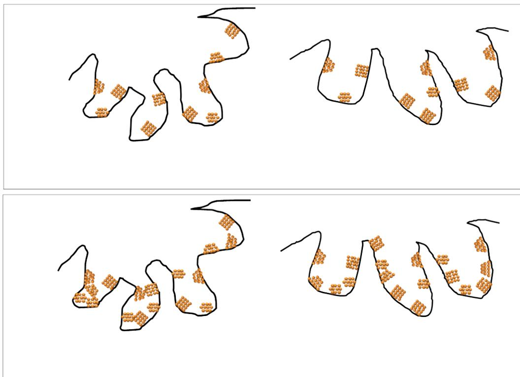
Schematic illustrations highlighting the pore size accessibility as a function of the cobalt loading on the two types of SiC carriers. (A) Low cobalt loading (10 wt. %) and (B) High cobalt loading (30 wt. %).
