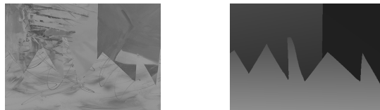
Figure 4. The photometrically adjusted left image and the true disparity map of the Sawtooth Stereo Image Pair .
