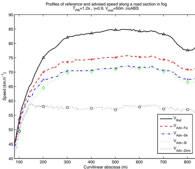
Fig. 12. Different speed profiles in fog with  $V_{Met} = 50$  m.
