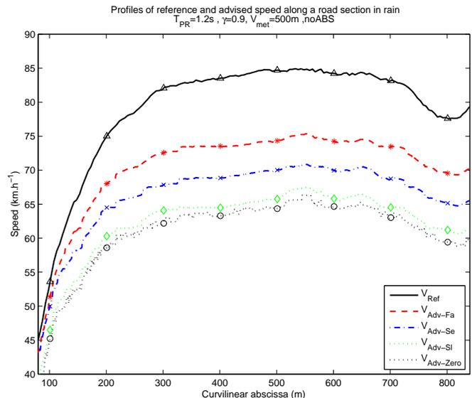
Fig. 9. Profiles of advised speeds computed with different safety criterions on wet road.
