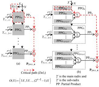
Fig. 1. Generalized  $N \times N$  bit radix-2<sup>r</sup> parallel multiplier.
