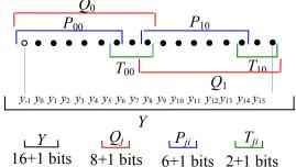
Figure 2. Partitioning of a 16-bit Y operand with r=8, s=6 and t=2
