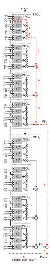
Fig. 4. Optimal partitioning of a two's complement  $64\times64$  bit radix- $2^{32}$  parallel multiplier based on equation (15) with (r,s)=(32,8).
