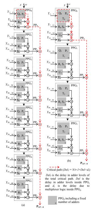
Fig. 2. Two's complement 64×64 bit multiplier.
