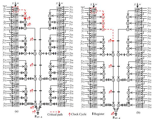
Fig. 5. Space/Time partitioning of a two's complement 64×64 bit radix-2<sup>32</sup> parallel multiplier based on equation (15).
