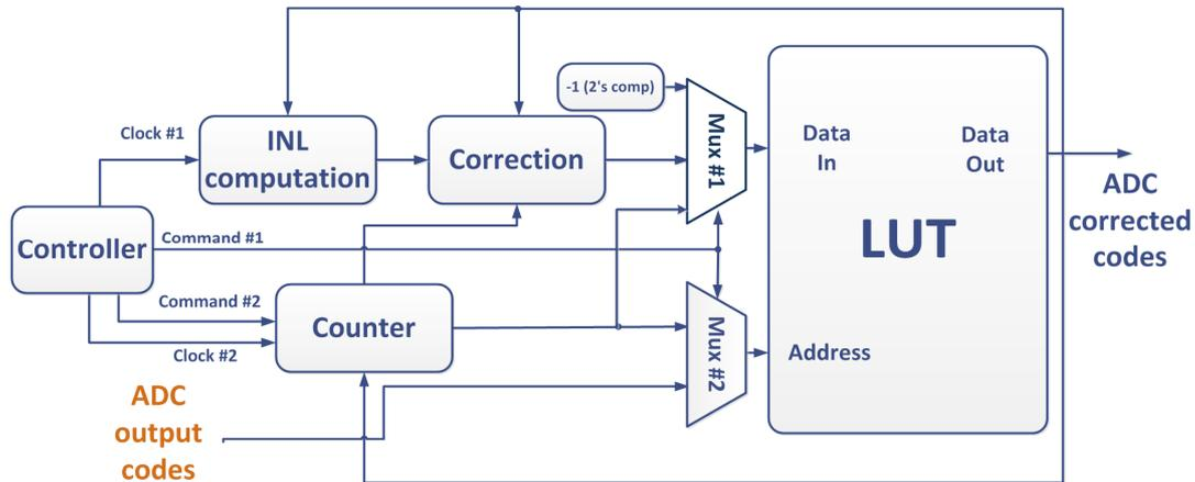
Figure 2 : hardware architecture for LUT computation
