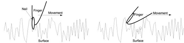
Figure 3: Left: A nail which is scratching a surface. Right: A finger which is rubbing a surface (asperities which are not "seen" by the finger are circled). For clarity, dimensions of the asperities are exaggerated on the scheme.
