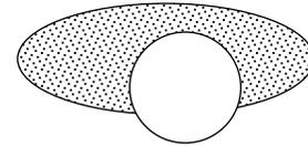
Fig. 15. Each particle is modeled by an ellipse and a circle, representing the top-view of the shoulders and head, parametrized as in eq. (31)
