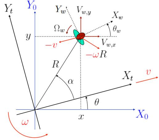
Fig. 3. Frames and variables definition for the *CyberCarpet*
