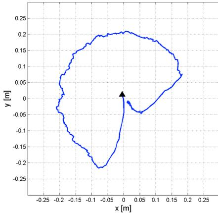
Fig. 26. Absolute trajectory in the experiment of Sect. VII-C.1 (circular path, with pure feedback control)
