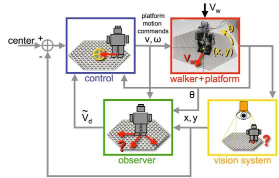
Fig. 2. Control system architecture of the *CyberCarpet*
